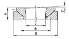
$\begin{array}{ll} D & = 80 \\ d & = 44 \\ d1 & = 61 \\ H & = 20 \\ Max \ screw \ dimension = M36 \\ Static \ load \ (kN) & = 323 \\ Weight \ (g) & = 427 \end{array}$
